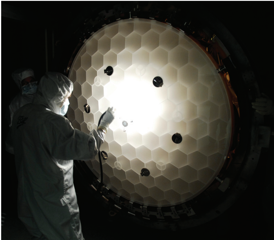
Inspection of the 1.4 meter primary mirror honeycomb structure. The mirror has been 86% light weighted, and only weighs 14% of a solid mirror of the same dimensions.
